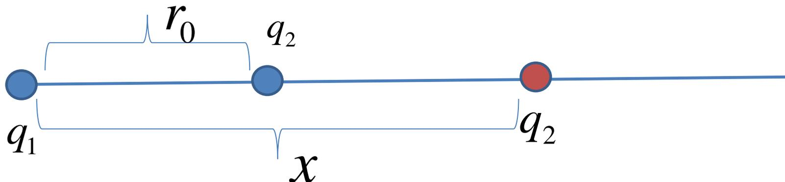
$$\varphi = q_2 \int_{r_0}^{\infty} \frac{q_1}{4\pi\epsilon_0 x^2} dx = \frac{q_1 q_2}{4\pi\epsilon_0 r_0} = q_2 \varphi_{12}$$
